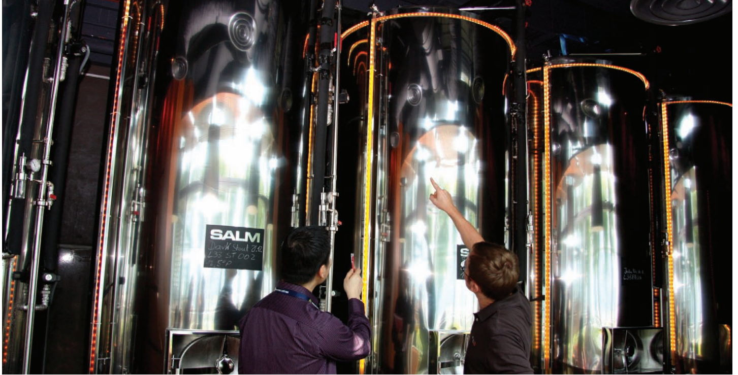
After one to two weeks, the beer is ready and transferred from its fermentation tank (pictured above) to the dispensing tank. At this point, the quantity of beer produced is declared to Singapore Customs for duty payments.
